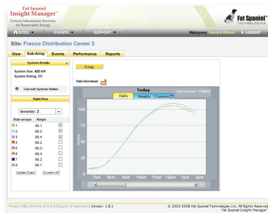
Fat Spaniel sub-array monitoring Web view.
